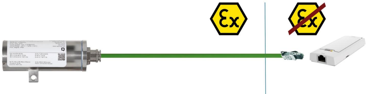
Figure 5-4 ExCam IPP1275 → safe area
