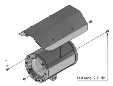
Figure 6-1 Removing the weather protection roof
