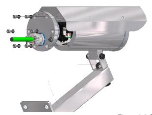
Figure 6-2 Opening ExCam miniTube IP
