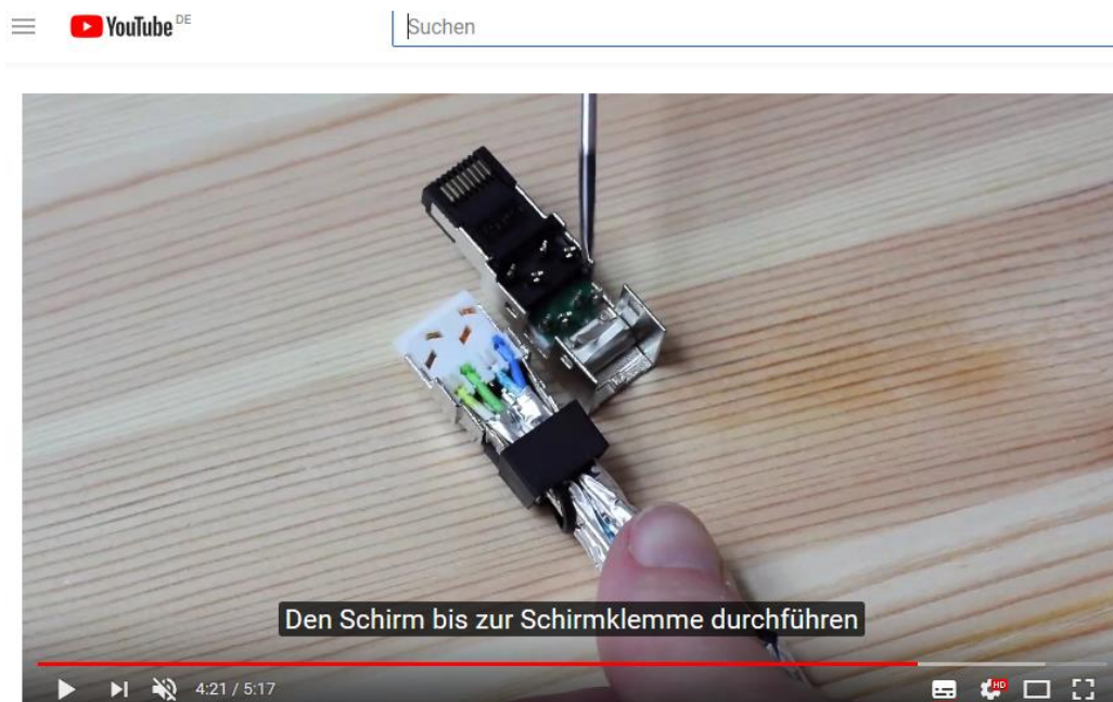
Figure 5-8 Plug assignment, RJ45
