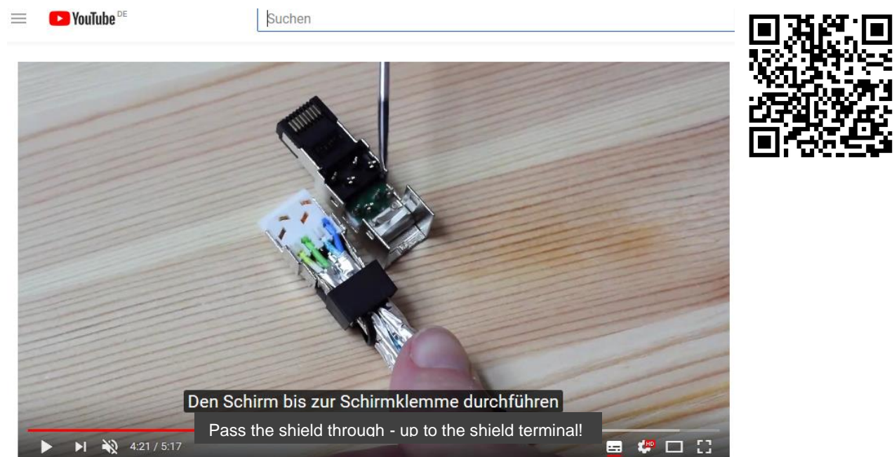
Fig. 5-8 Plug assignment, RJ45
