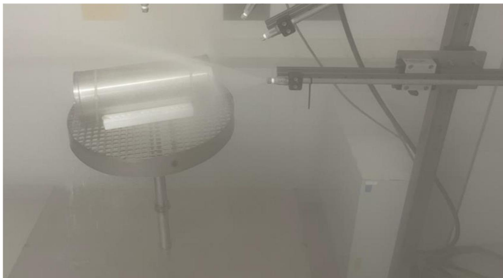
Fig. 16: Test specimen 003 before and during the steam jet test IPX9K
