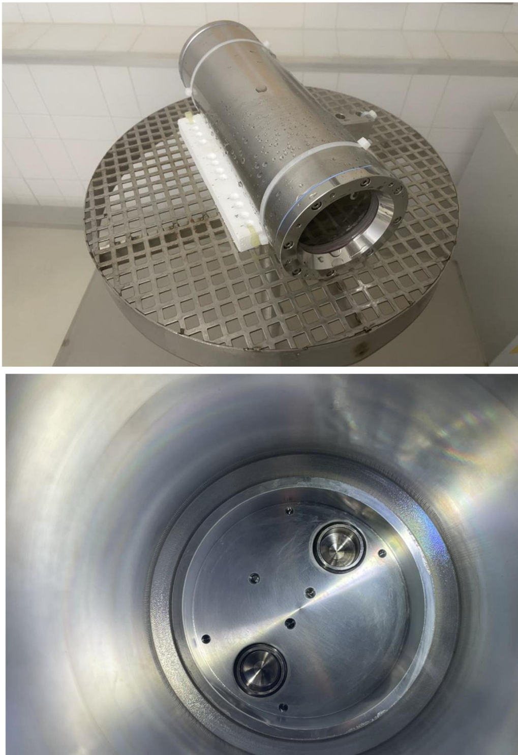
Fig. 14: Test specimen 002 after the steam jet test IPX9K - no water ingress
