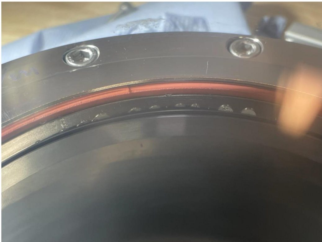
Fig. 20: Test specimen 004 after the steam jet test IPX9K - no water ingress inside the enclosure; water accumulation between outer red and black seal
