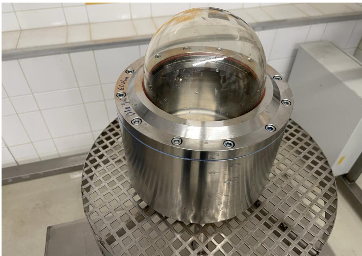
Fig. 8: Test specimen 004 before the strong water jet test IPX6
