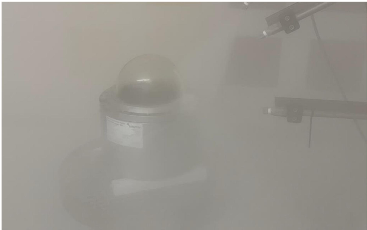
Fig. 19: Test specimen 004 before and during the steam jet test IPX9K
