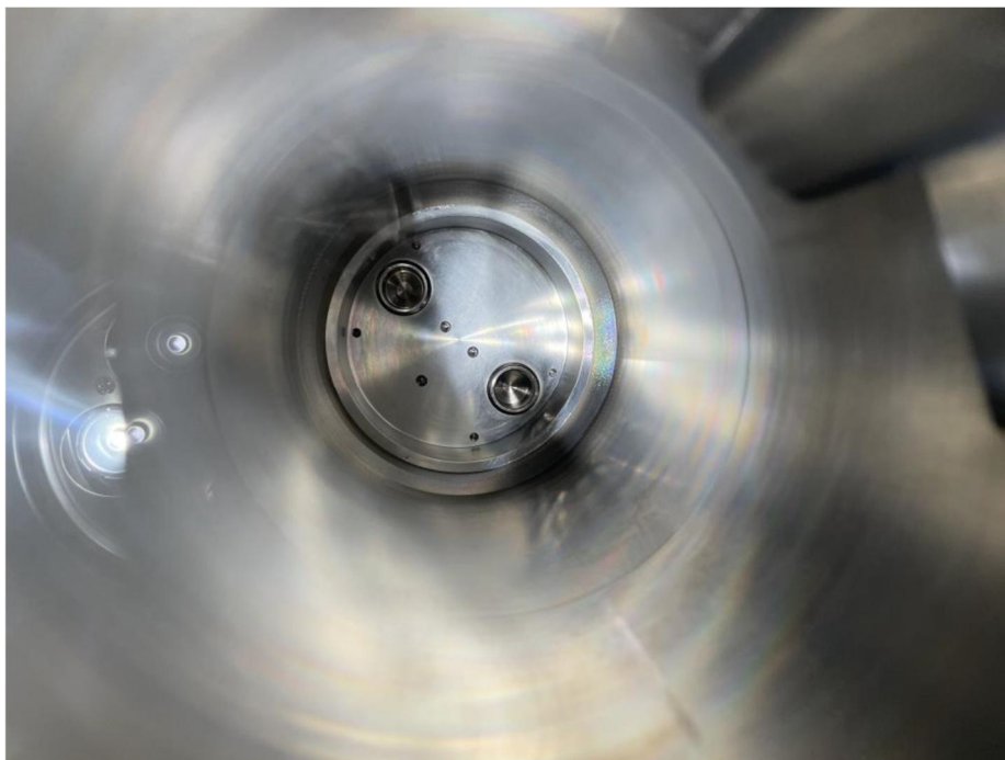
Fig. 5: Test specimen 002 after the strong water jet test IPX6 - No water ingress
