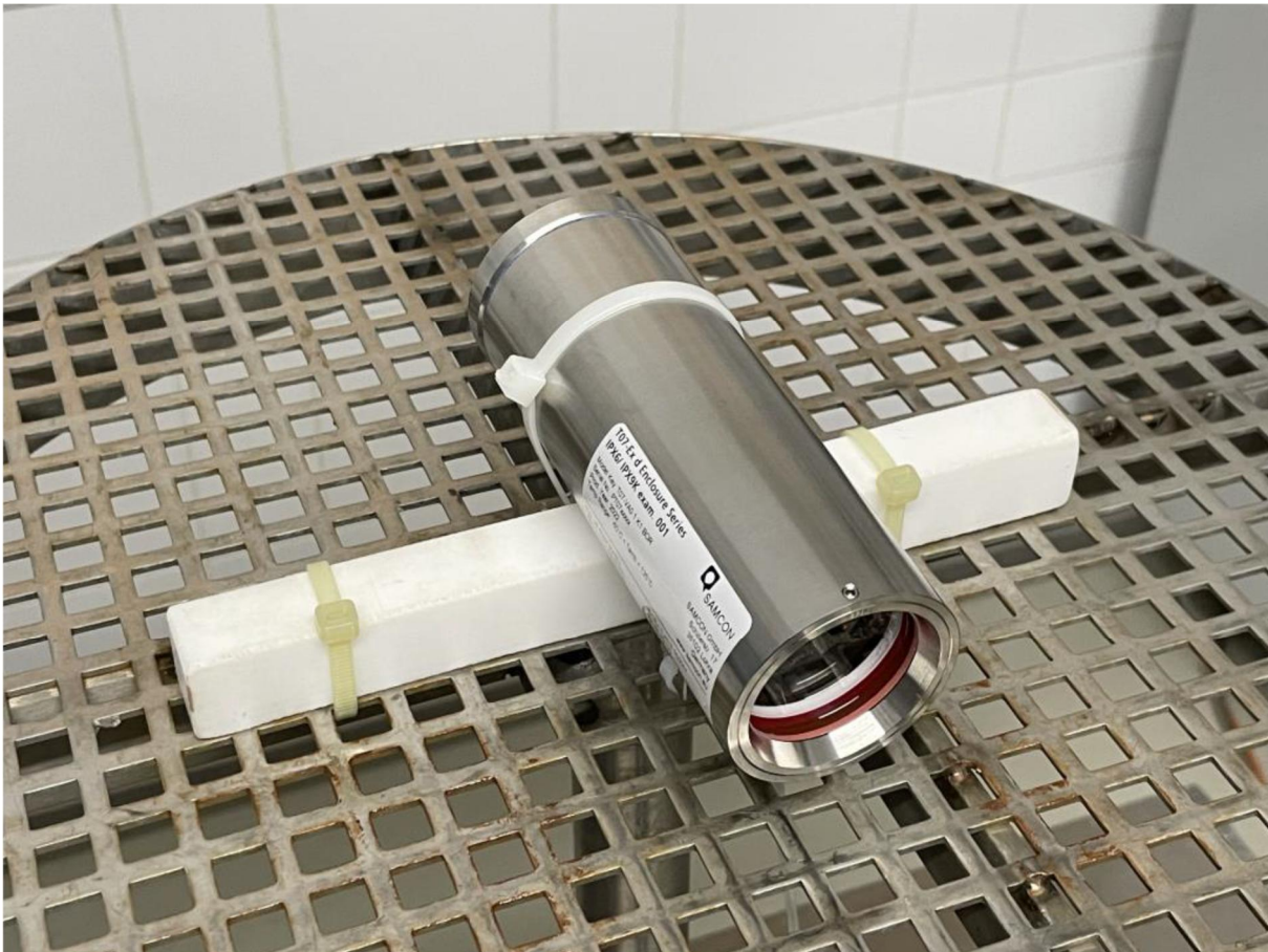
Fig. 2: Test specimen 001 before the strong water jet test IPX6
