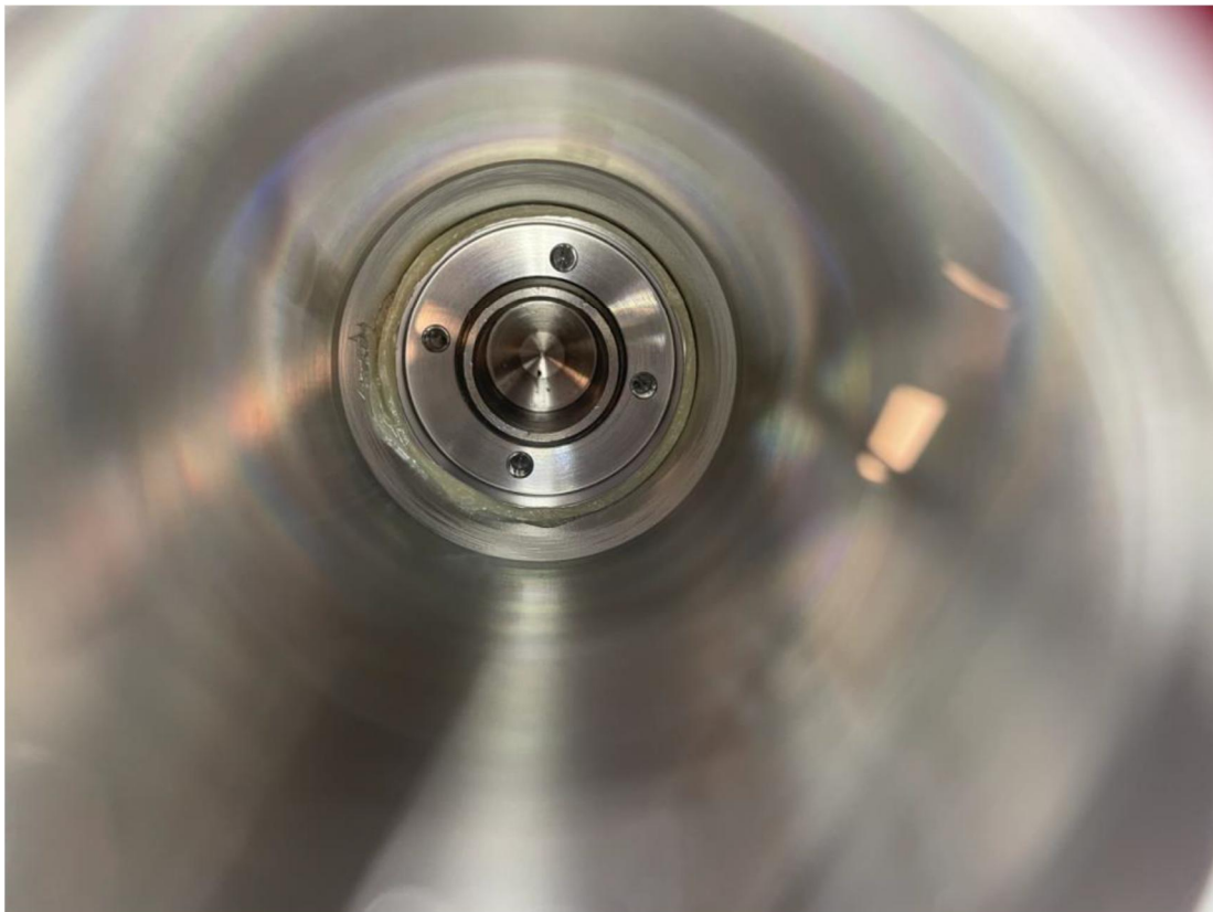
Fig. 11: Test specimen 001 after the steam jet test IPX9K - no water ingress
