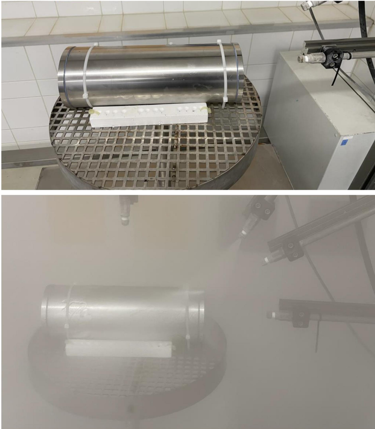
Fig. 13: Test specimen 002 before and during the steam jet test IPX9K
