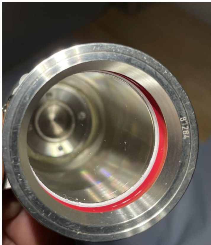
Fig. 3: Test specimen 001 after the strong water jet test IPX6 - No water ingress
