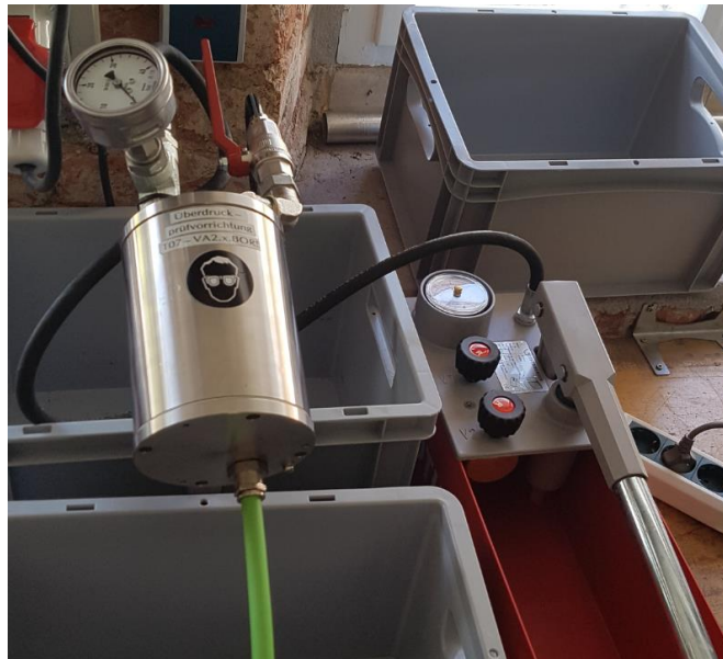
Fig. 2-3: Pressure testing devices for cable and cable gland combinations
