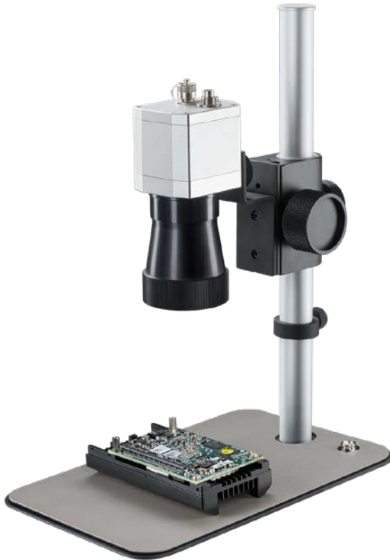
Microscope optics PI 640 for the inspection of PCBs
